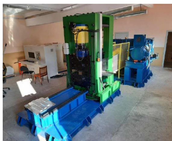
Fig. 1. General view of reversing mill DUO 400 sheet rolling mill with individual drive of working rolls
