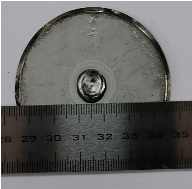
Fig. 7. Ion beam imprint on stainless steel after prolonged exposure
