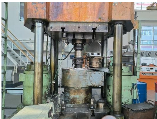
Fig. 2. High pressure torsion equipment diagram
